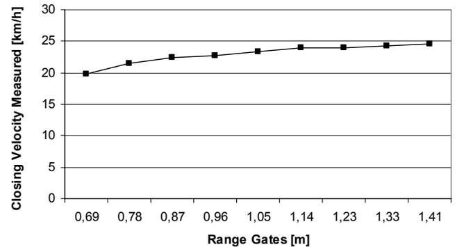
**Figure 12: Doppler measurements at discrete distances**
