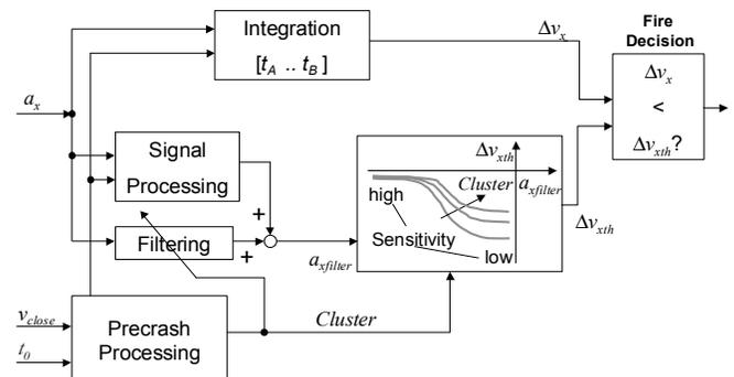
**Figure 5: Algorithm block diagram for a single sensor configuration ( $v_{close}$  = closing velocity,  $t_0$  = time to expected impact)**
