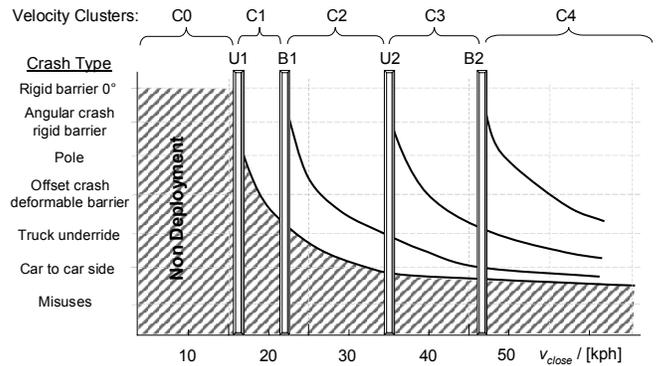
**Figure 3: Clustered crash set with thresholds separating the required set of restraints**
