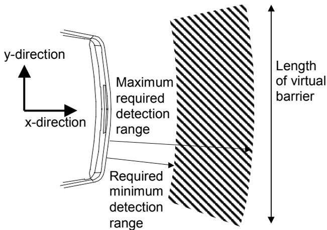
**Figure 1: Virtual barrier at vehicle front and vehicle coordinates**
