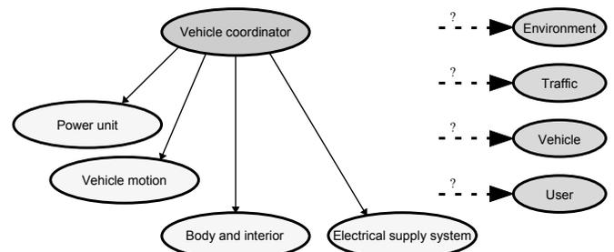
**Figure 7: CARTRONIC® structure for the complete vehicle systems (first level)**
