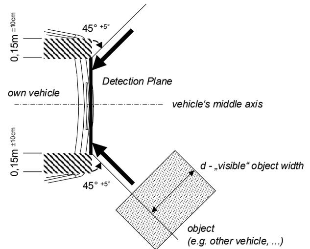
**Figure 2: Definition of frontal crash for PRESET and PREFIRE by definition of a detection plane on the vehicle surface**
