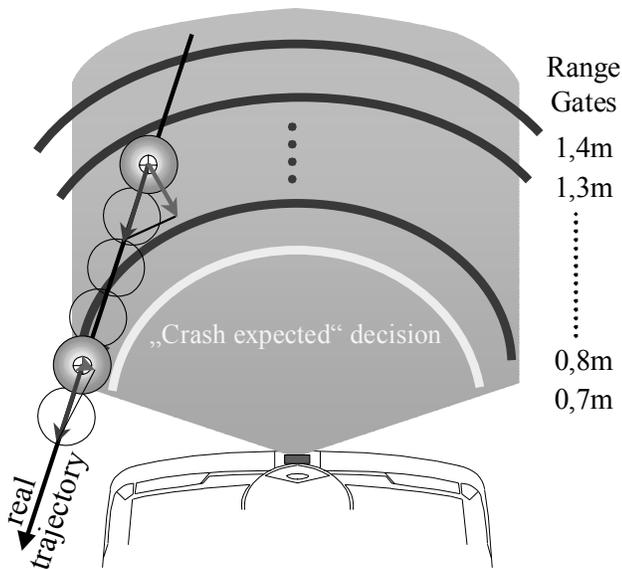
**Figure 8: Closing velocity measurements during Doppler mode for single sensor configuration**
