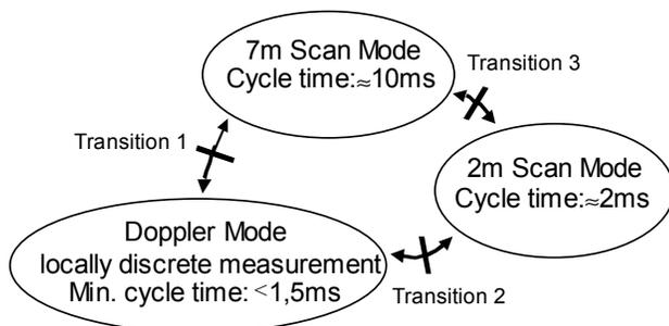
**Figure 9: State diagram with sensor measurement modes and transitions**
