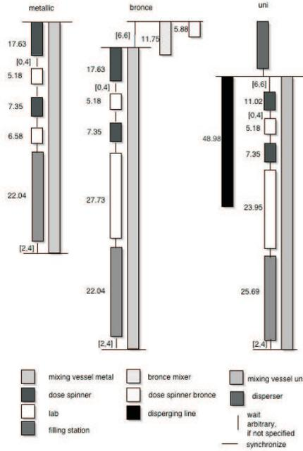
Figure 2: Recipe-based representation of the production sequence.
