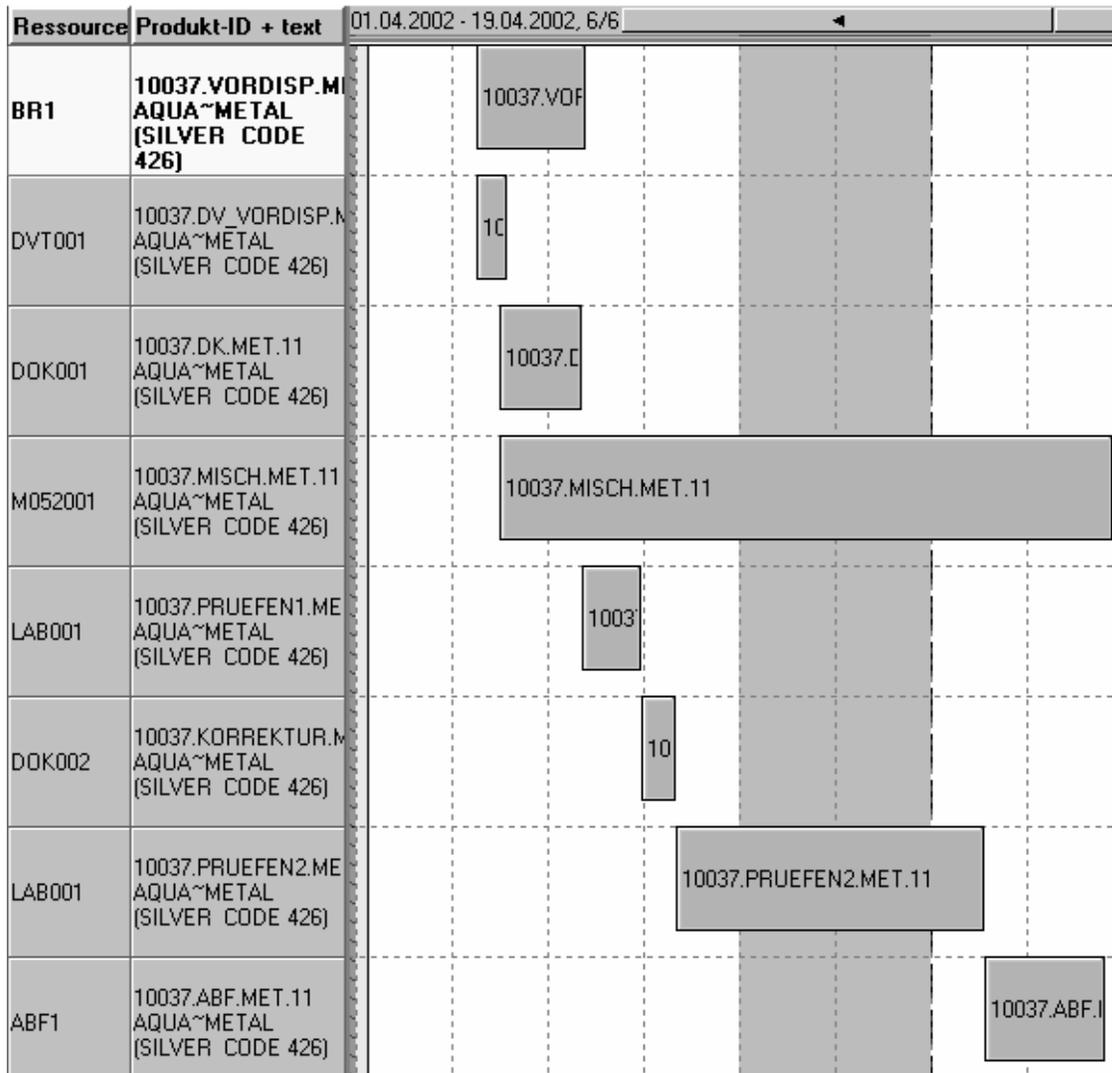
**Graphic 6: Example for a resource assignment when producing special metallic lacquers**
